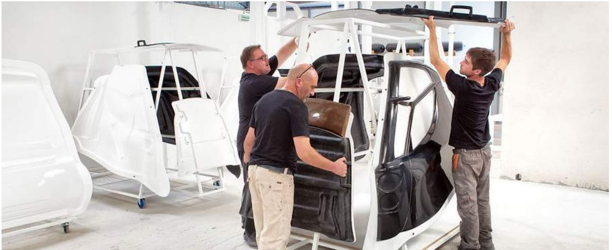
Installation of the body elements on the shaper
