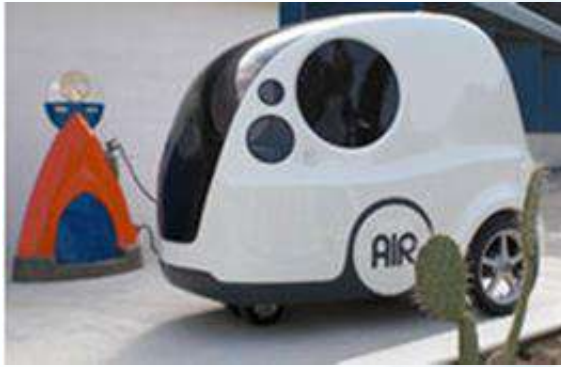
Caption: The multiple options for refilling the MDI vehicles is a big advantage, especially via the filling station or the mobile facility. When combined with the dual energy mode travel autonomy becomes attractive and competitive.
